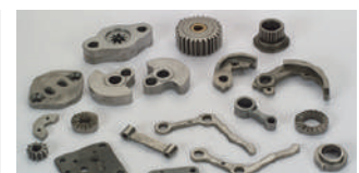
▲ Powder Metallurgy: Preparation of metal materials, composite materials, and other material systems. Applications include ceramic materials such as turbine blades and engine components, wear-resistant parts like brake pads and clutch plates, as well as biocompatible materials for implants and other medical devices.
